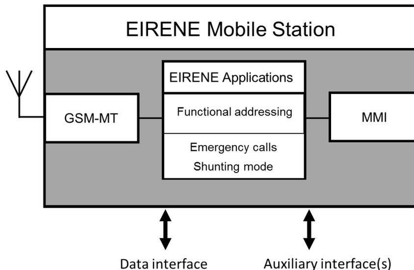
Figure 7A-1: Logical Shunting radio architecture and interfaces
