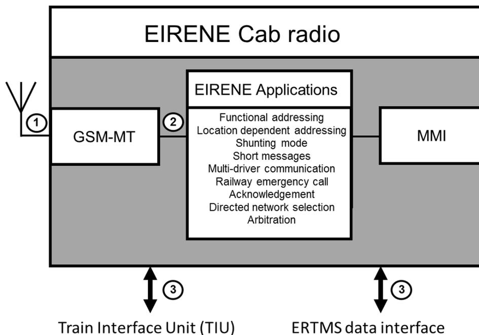
Figure 5-1: Logical Cab radio architecture and interfaces
