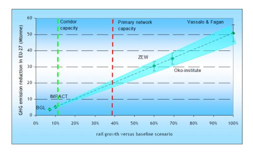
The graph demonstrates the possible CO2 reduction achievable in the EU through an increase in rail freight and a corresponding decrease in road freight in the EU by 2020, under different scenarios.
