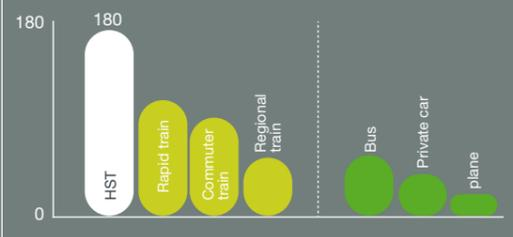
Due to high speed rail's very high transport capacity, the land needed for the large traffic volumes carried is much reduced.
