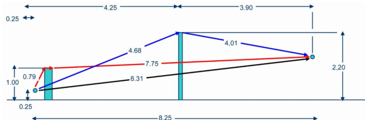
Figure 12: Geometric comparison of low height barrier close to rail with the usual configuration at about 4 m. The noise reduction is about the same in both situations.
