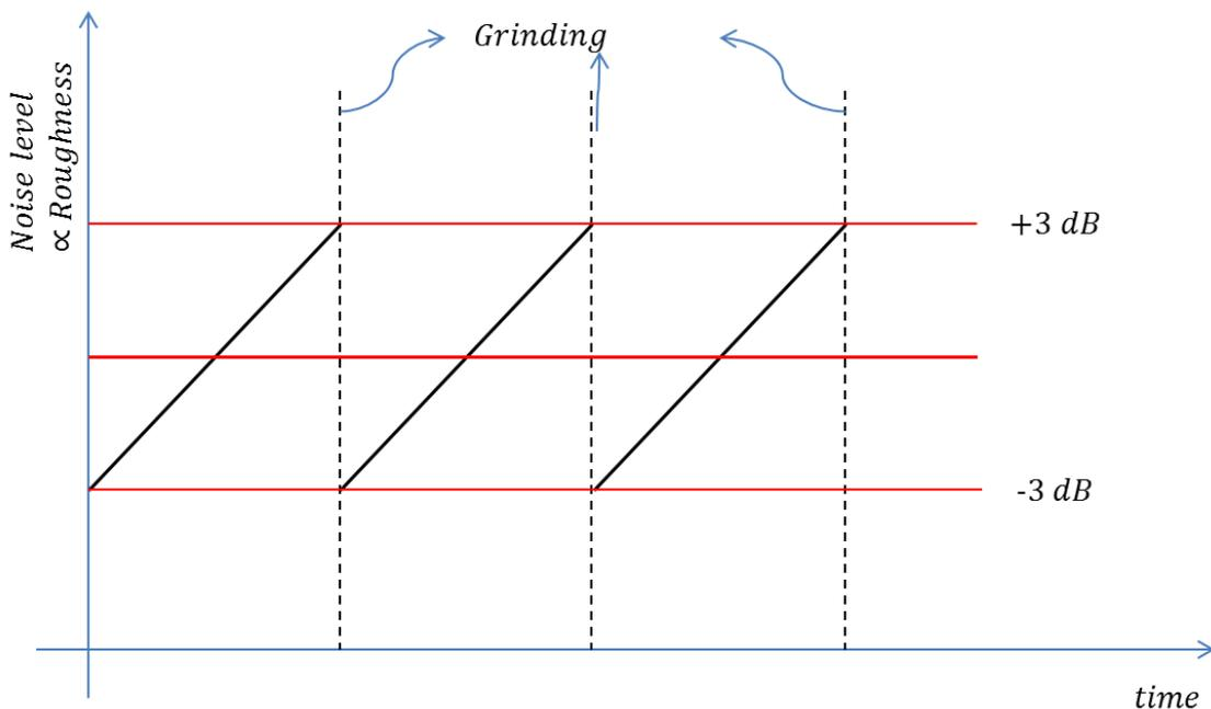
Figure 10: Evolution in time of the rail roughness by applying acoustic grinding procedure. In this model linear grow of roughness and proportionality between noise and roughness are assumed. The BÜG procedure in Germany is based on this model and grinding is done when the noise level is exceed by 3 dB.
