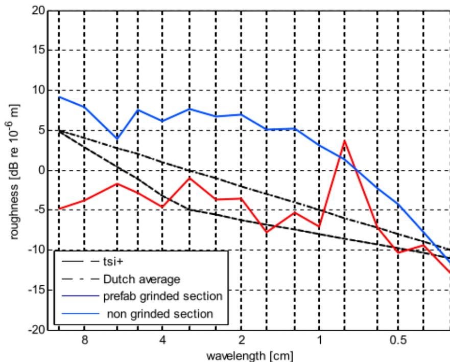
Figure 4: Example of roughness spectrum (Figure from M+P Report<sup>2</sup>).
