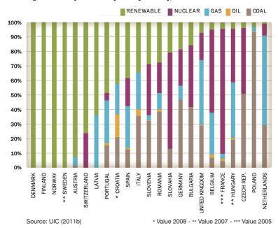
Fig.27: Railways electricity mix, 2005 inside - 2009 outside
