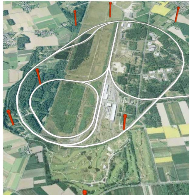
Figure 2: Illustration of the railGATEs pseudolites, © RWTH/IRT
