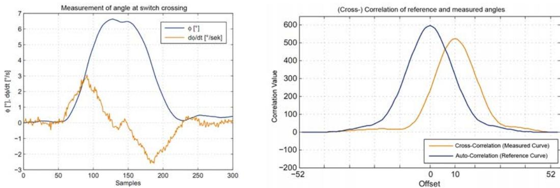
Figure 3 Detecting switches via gyroscope measurements and subsequent correlation.
