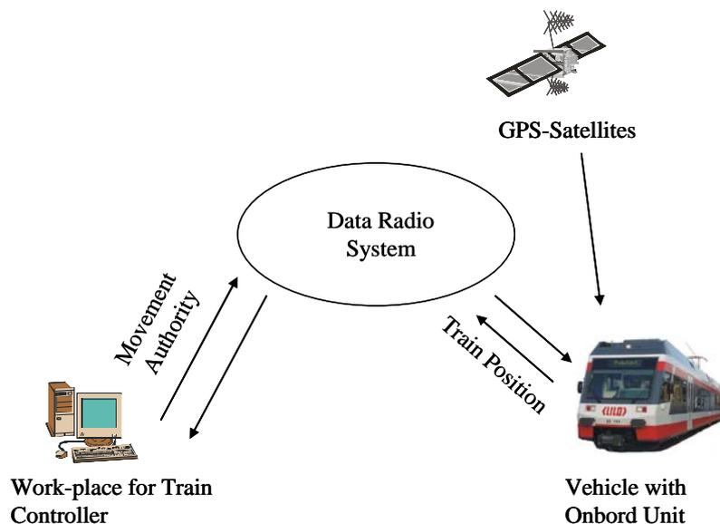
Figure 1 Schematic overview of the TCS.
