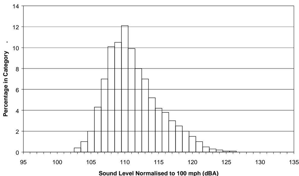
**Figure 9: Distribution of Underfloor A weighted Sound Pressure Level Normalised to 100 mph**
