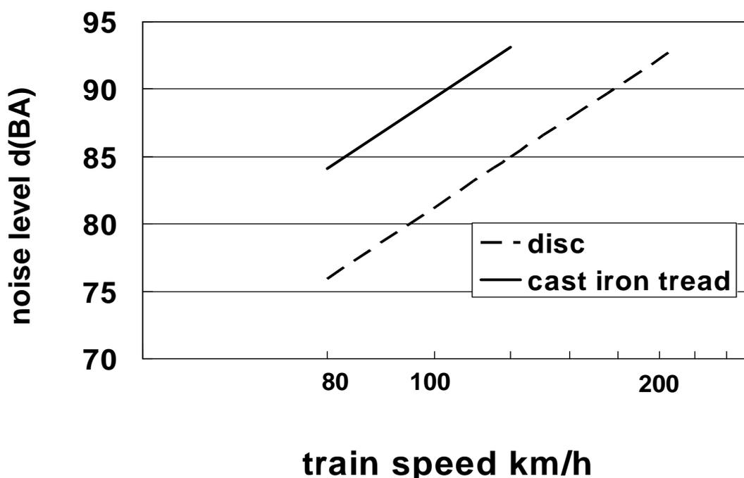
**Figure 5 Effect of Train Speed and braking system**
