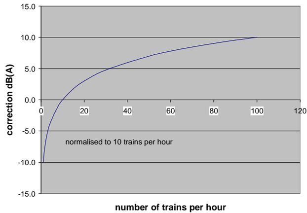
**Figure 7 : correction for number of trains per hour**
