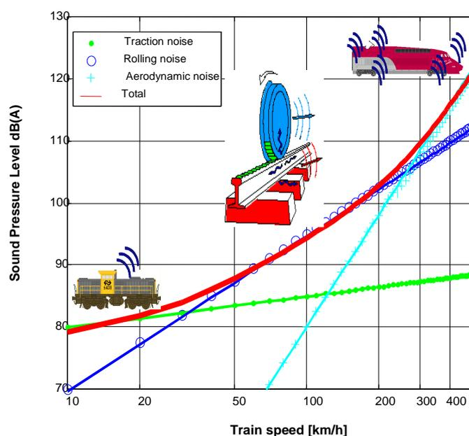
Figure 2. : Sound pressure level as a function of train speed
