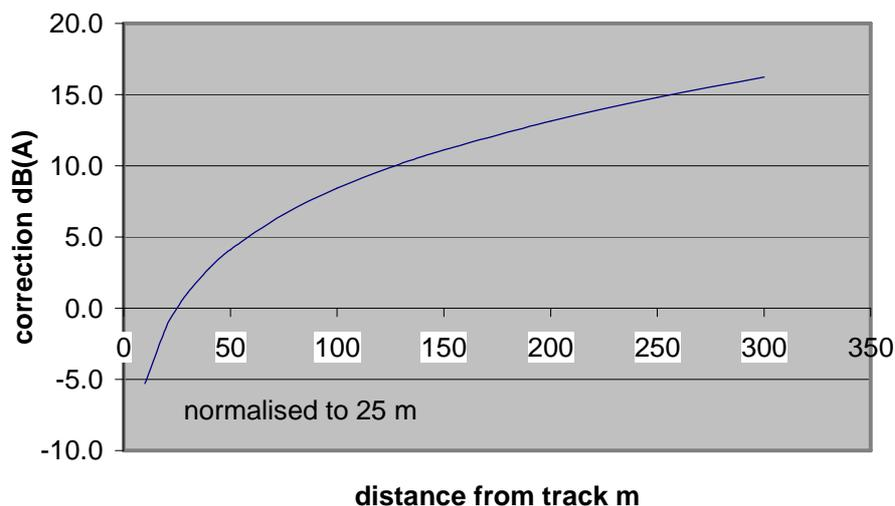
**Figure 8 : reduction of train noise energy with distance**
