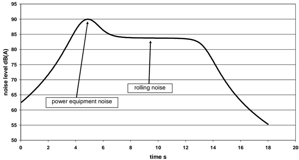
**Figure 3 : noise level time history for diesel hauled train (80km/h, d = 25m)**
