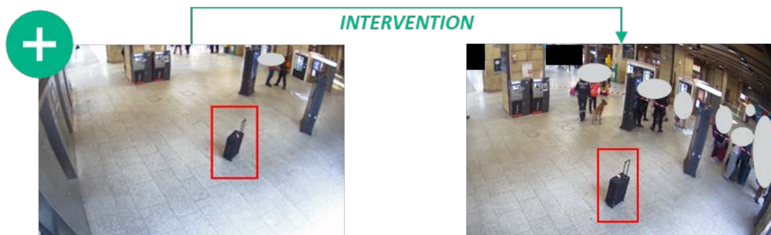
Figure 31 - Successfully initiated intervention procedure triggered by an abandoned object alert
