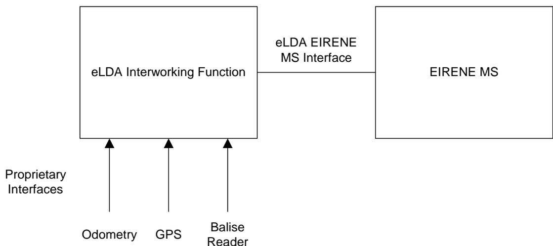
Figure 2-3 Train based architecture
