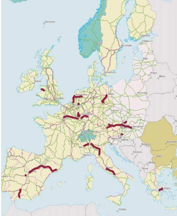
Commercial lines equipped with ETCS by the end of 2008
