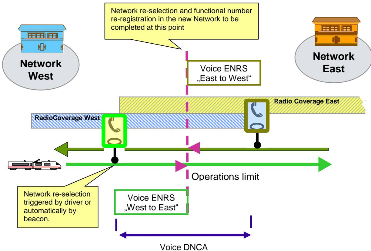
Figure 1: Dual Network Coverage Zone at EIRENE network borders without ETCS)
