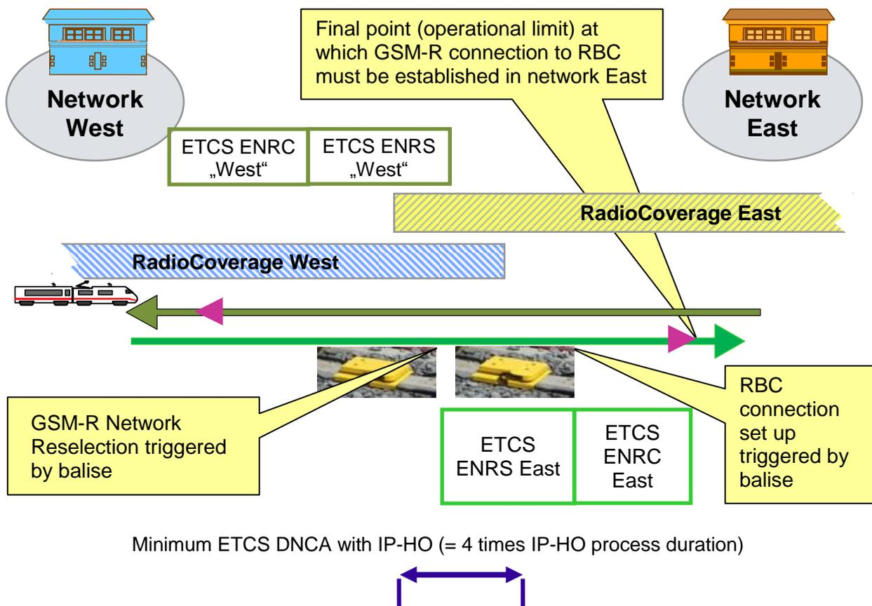
Figure 4: Minimum DNCA including ETCS and use of IP-HO
