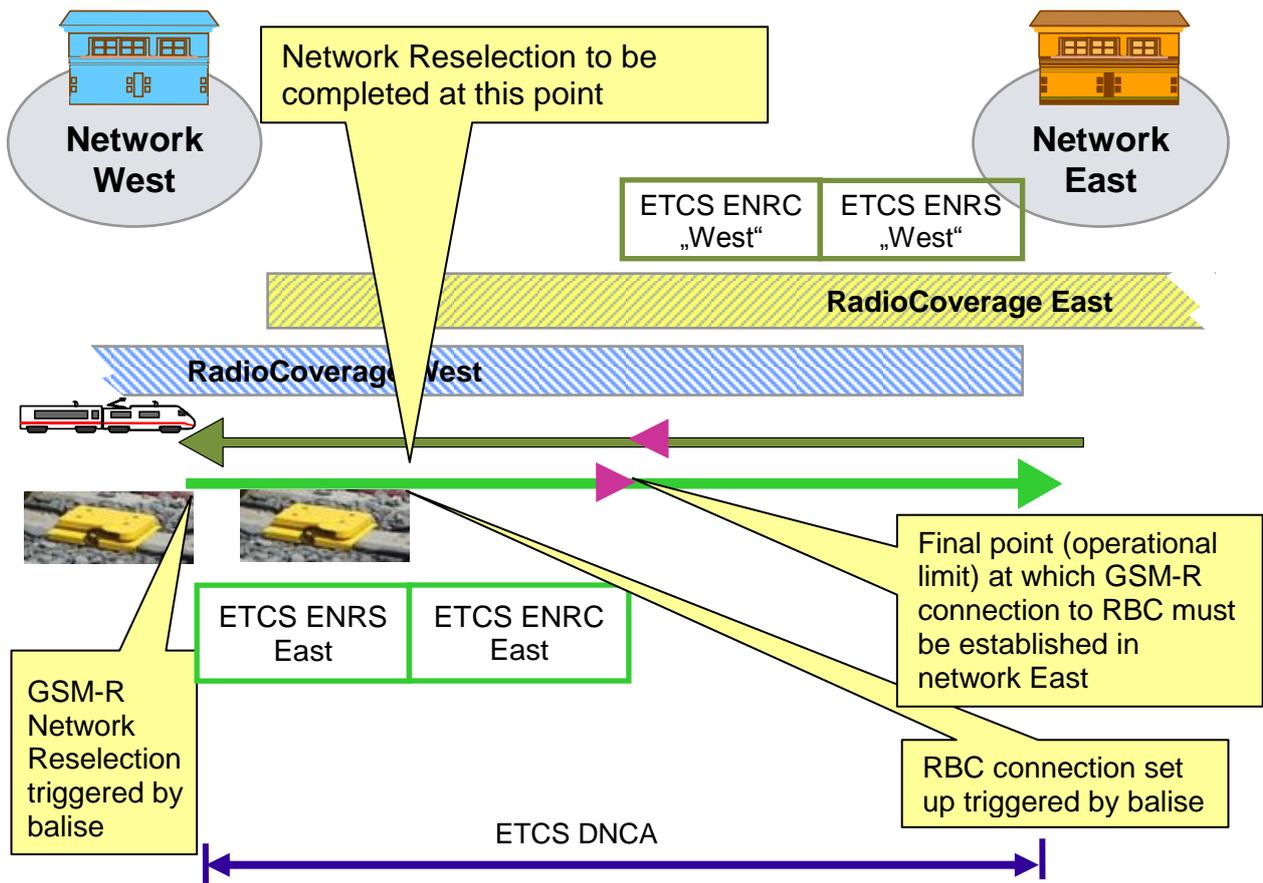
Figure 2: Dual Network Coverage Zone at EIRENE network borders including ETCS
