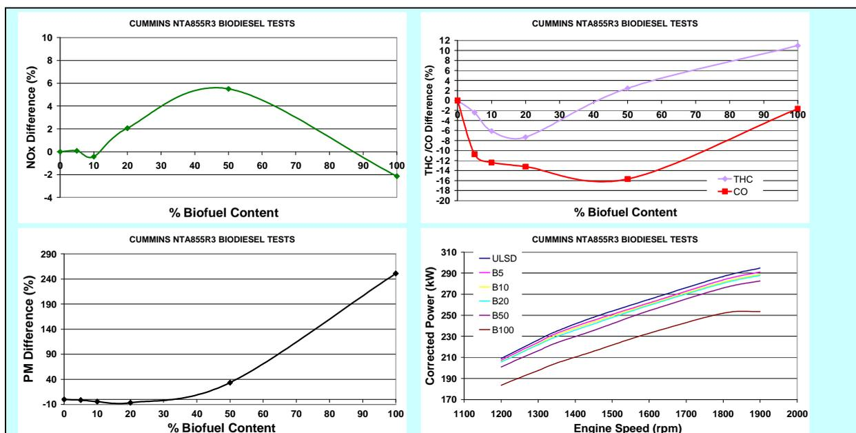
**Figure 1: Initial results of UK bench trials of Biodiesel with the Cummins NTA855R3 engine, [Results are presented as % changes relative to ultra-low sulphur diesel fuel.]**
