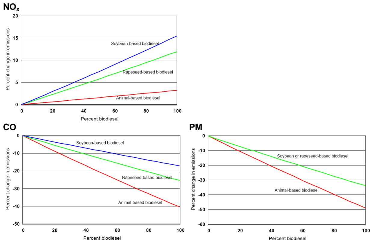
The US EPA study does also highlight that there can be important differences in the relative emissions performances of Biodiesel produced from different source oils, as illustrated in Figure 18. It could be expected that such variation will be somewhat reduced as a result of the definition of Biodiesel standards, such as the European Standard EN 14214 for Biodiesel produced from vegetable oils.
