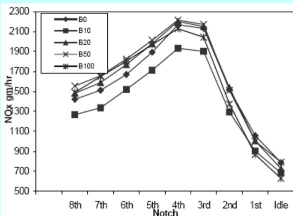
**Figure 2: NOx emissions for Biodiesel blends**
