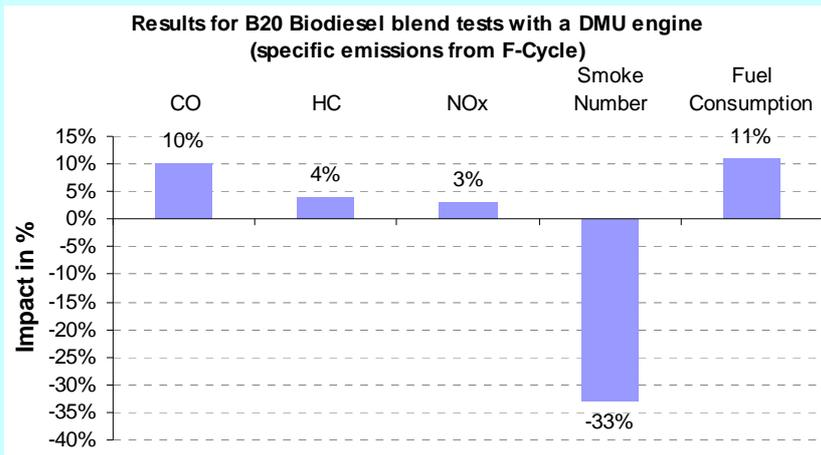
**Figure 1: Biofuel test results (80% diesel and 20% Biodiesel) relative to diesel, DMU engine**
