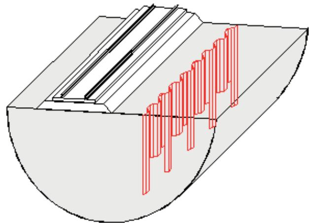
Graph 31. Construction of a sheet piling wall (left) and diagram of the construction of the wall (right). © Trafikverket.
