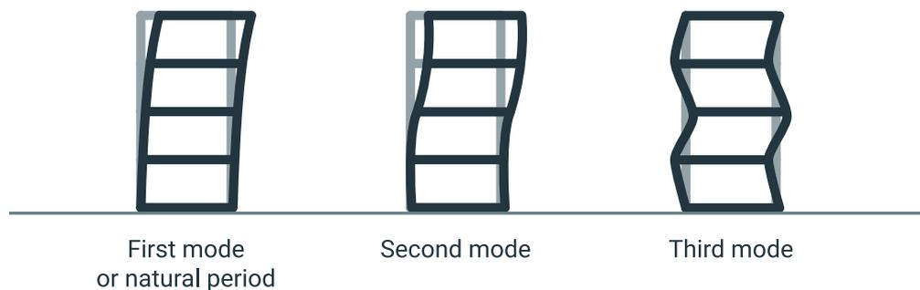
**Graph 7. Theoretical resonances of a building structure, first three modes with low frequencies (1 to 5 Hz, amplitude highly exaggerated). Higher modes result from the resonance of the floor spans [9].**
