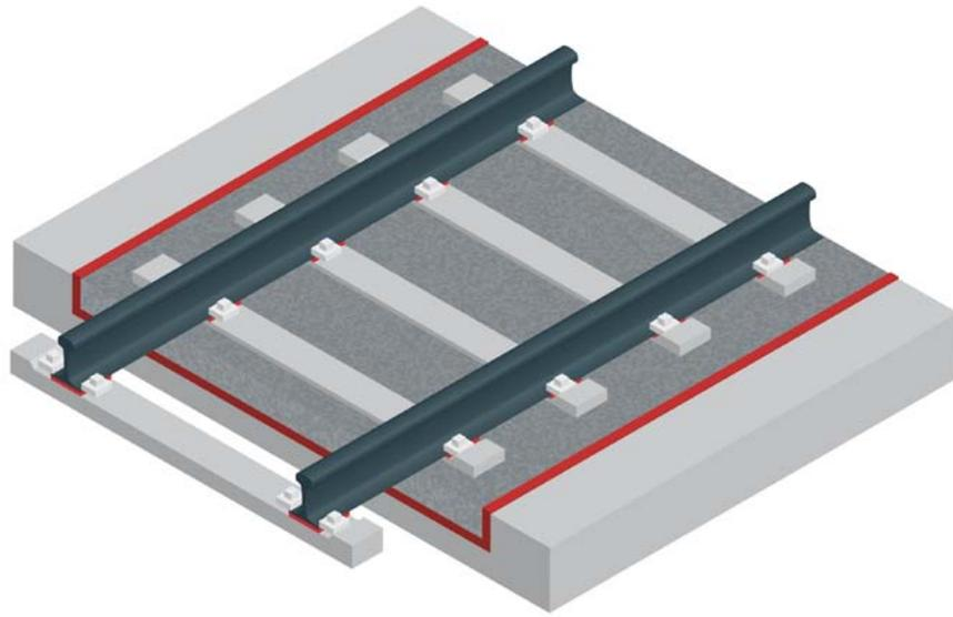
Graph 21. Under-ballast mat in a concrete trough or in a tunnel.
