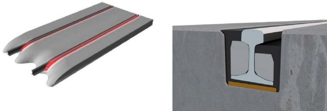
**Graph 17. Example of an embedded rail support in a concrete slab (right: Edilon Sedra; source: Wikipedia).**
