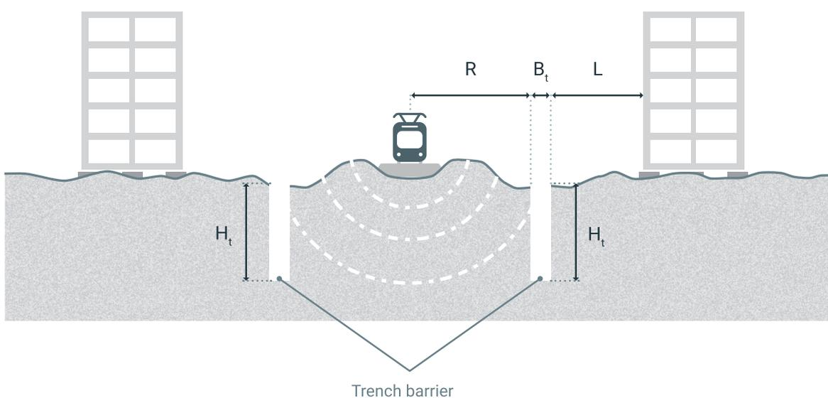
Graph 32. Example of a trench barrier – here for model calculation of its efficiency [42].
