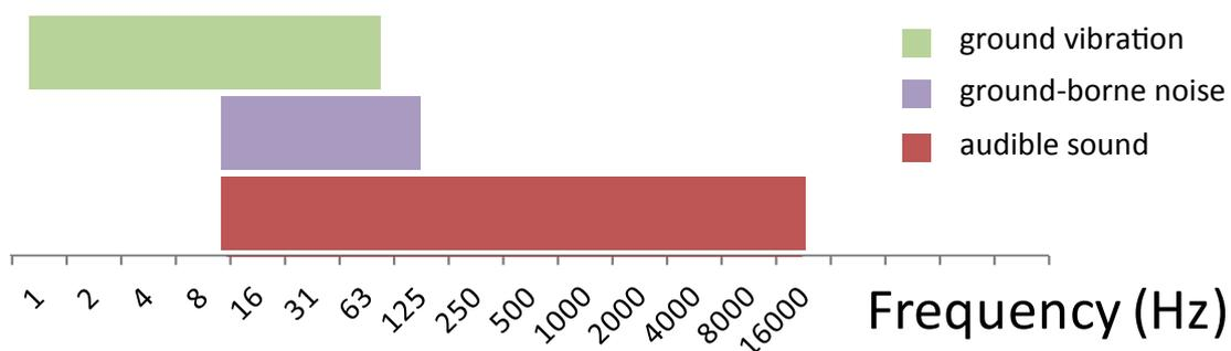
**Graph 5. Frequency ranges for audible sound, feelable ground-borne vibration and ground-borne noise.**
