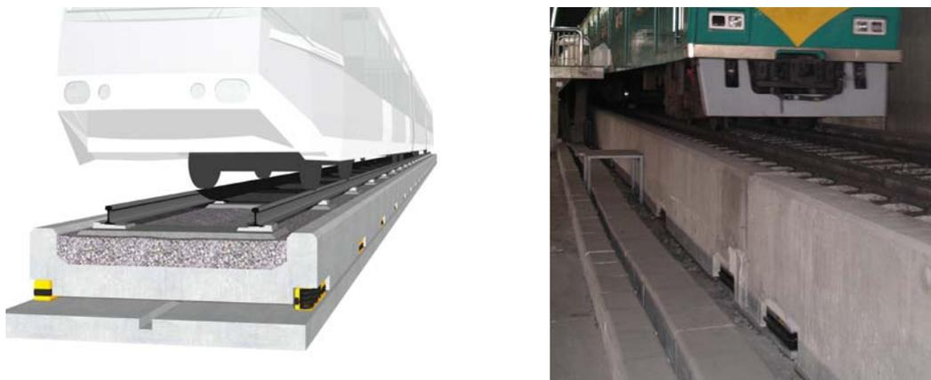
**Graph 29. Schematic of a mass spring system on steel coils (left) and real-life installation in a tunnel at Puchon Station, Korea. © GERB Vibration Control Systems.**
