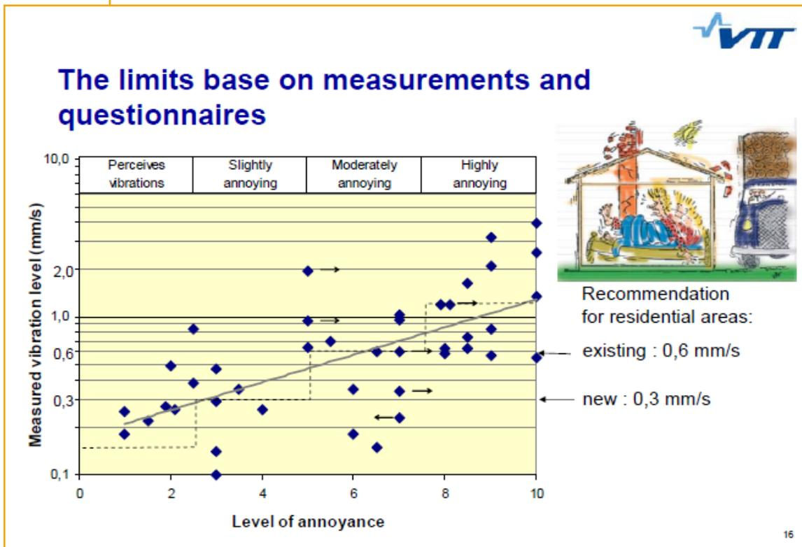
Graph 14. Illustration of recommended limit values derived from field survey and measurements (source: presentation by VTT).
