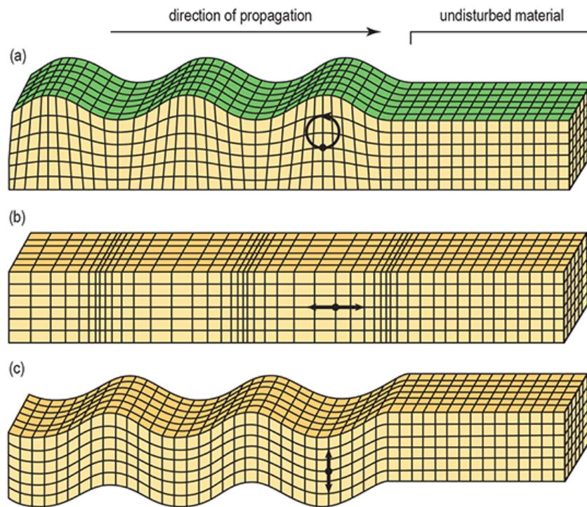
**Graph 6. The three main wave forms in the ground associated with the transmission of ground vibration [8].**
