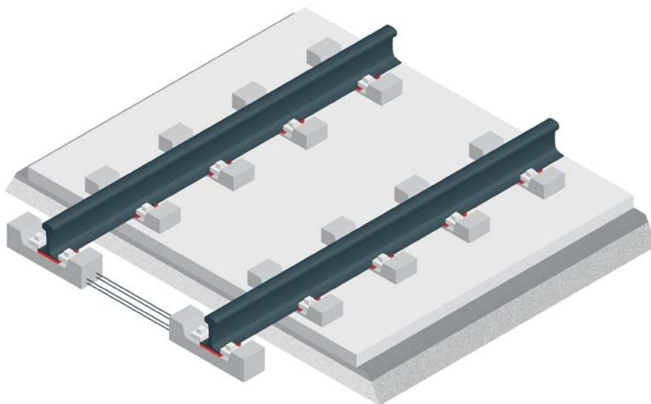
Graph 23. Non-ballasted track, with the rails being fixed in fixation blocks that are mounted on a concrete continuous slab (Rheda system).
