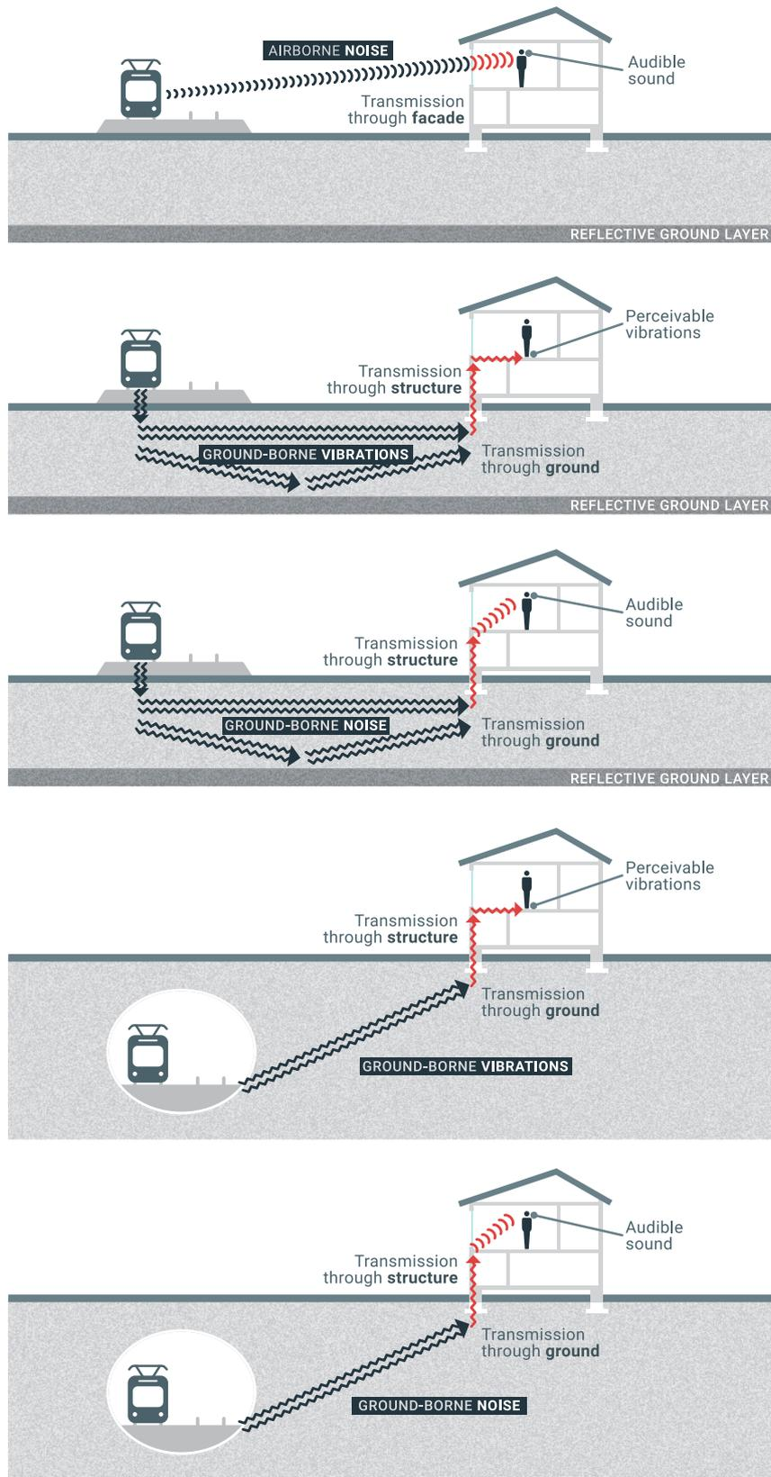
Graph 1. The different generating mechanisms and transmission paths of air-borne noise (not applicable for underground line), ground-borne vibration and ground-borne noise.
