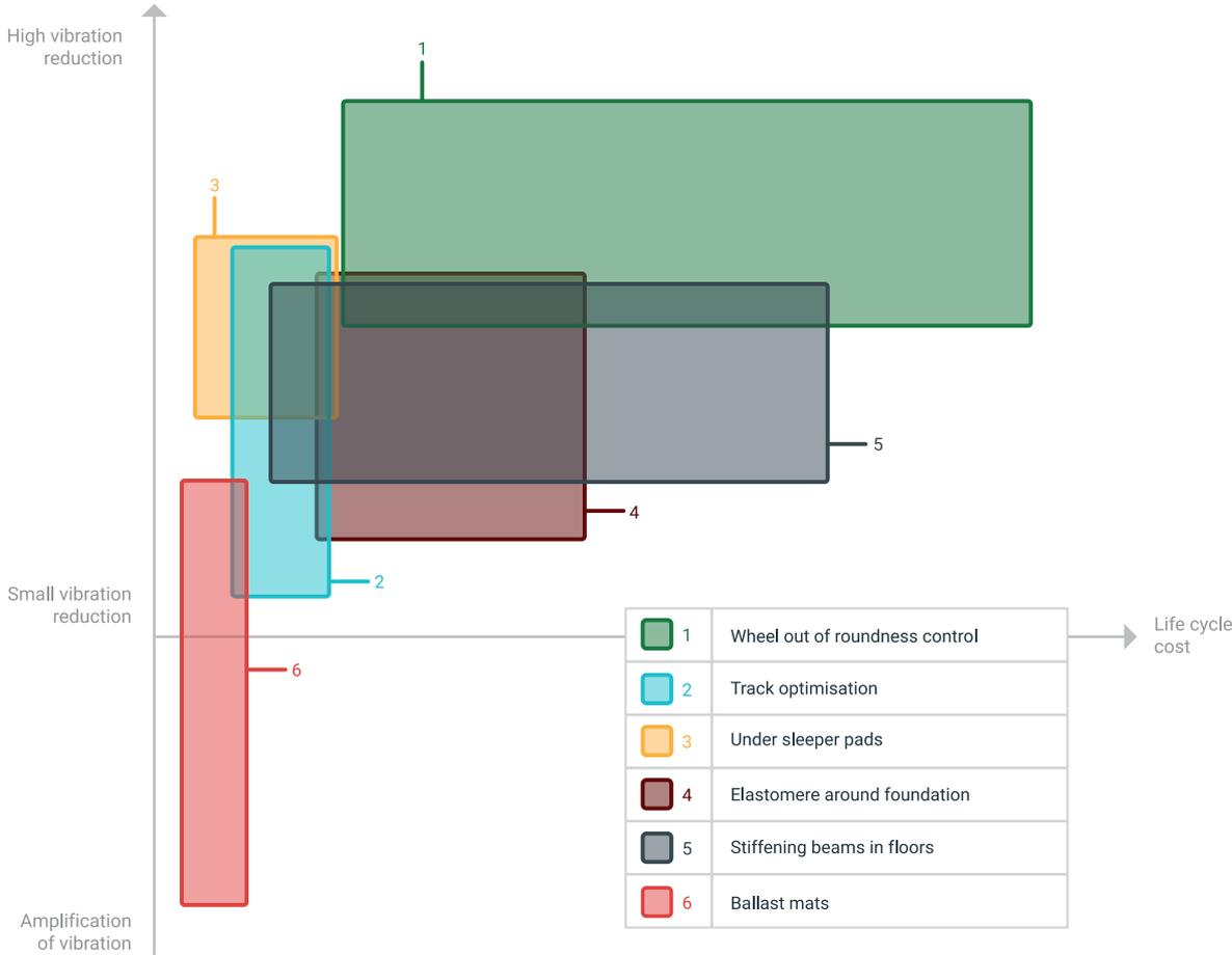
Graph 38. Comparison of mitigation measures suitable for application in existing tunnel situations. Annual simplified life-cycle cost for mitigation at a hot spot of 500 m length with 40 premises, and their effectiveness in terms of percentage reduced of the rms vibration velocity. A negative reduction means that there is a risk that the velocity will increase due to the measure being implemented.
