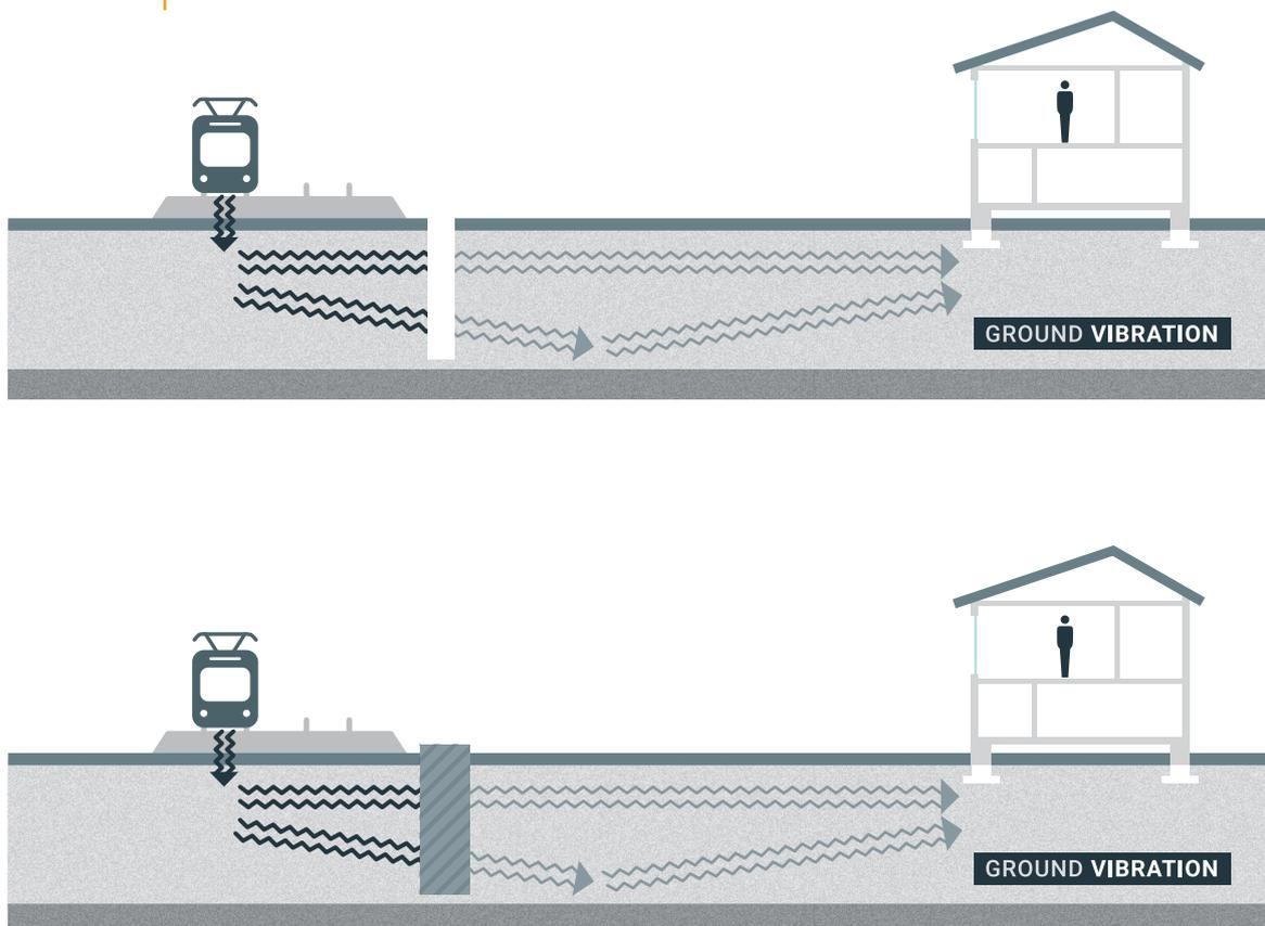
Graph 33. Schematic representation of a trench (upper graph) and a wave impeding block (lower graph).
