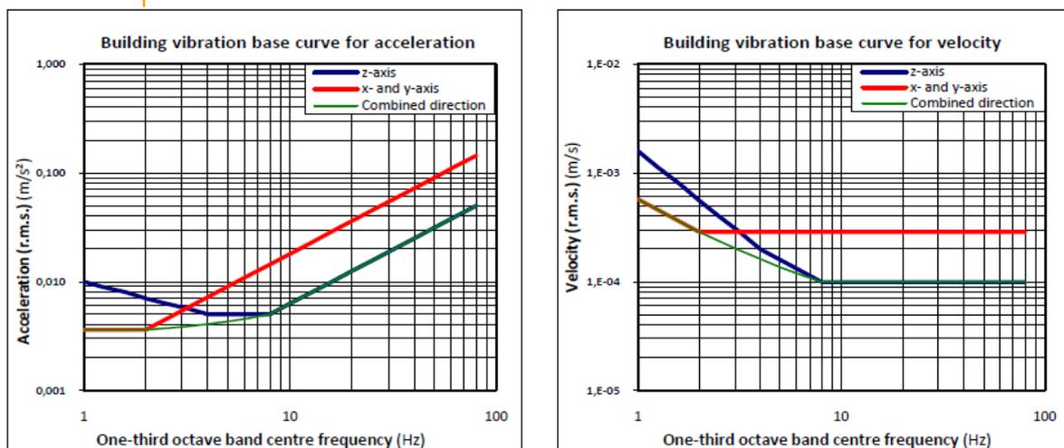
Graph 8. Building vibration base curves for just noticeable vibration expressed as acceleration (left-hand curve) or velocity (right-hand curve) for vertical and horizontal direction separately, as well as for the combined directions. After ISO 2631-2: 1989.
