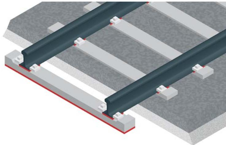
Graph 19. Under-sleeper pad for vibration reduction and ballast protection.
