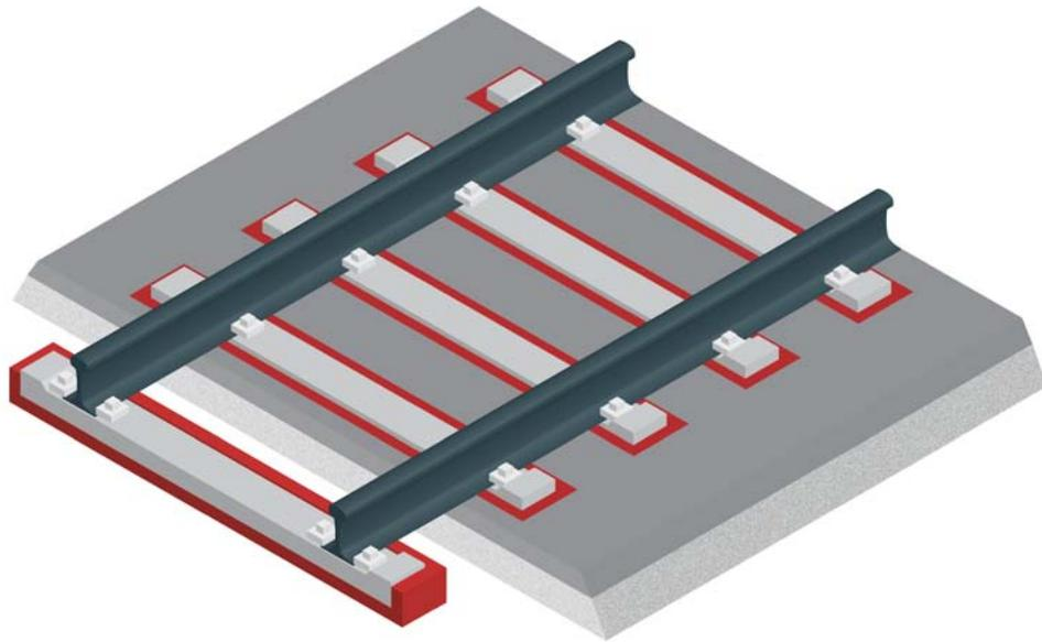
**Graph 26. Slab track lost in the subsoil, with under-sleeper mat to make it into a floating slab.**
