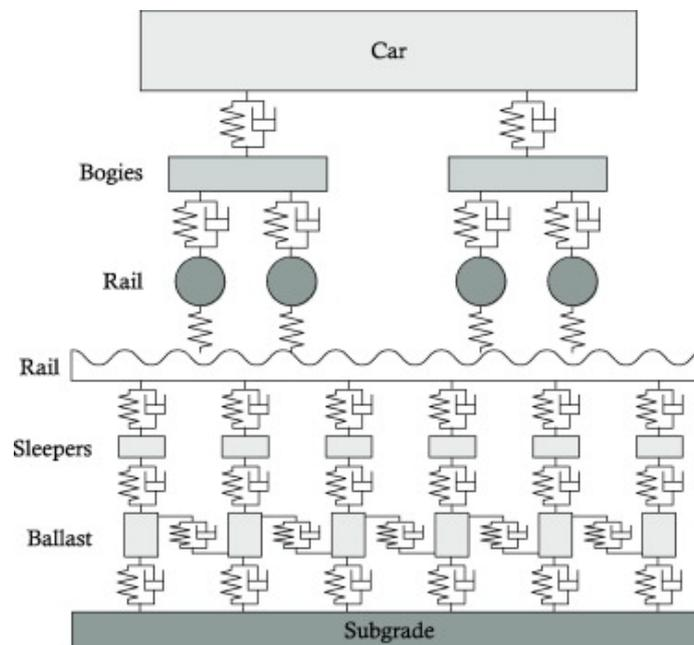
Graph 4. Schematic of the dynamic system of rail car, bogies, wheels, rails, sleepers and ballast on the subsoil [1].
