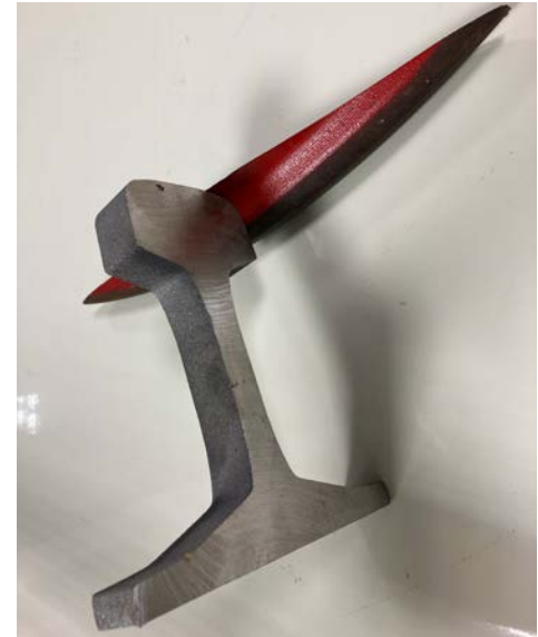
Rail and wheel flange cross-section – Coupe rail et boudin de roue UIC
