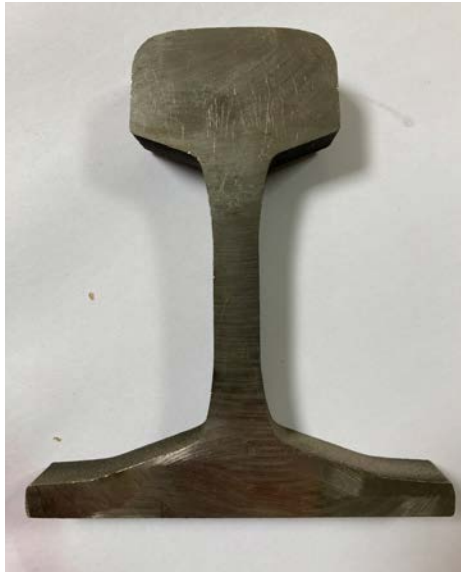
UIC 60 cross-section – Coupe UIC 60
