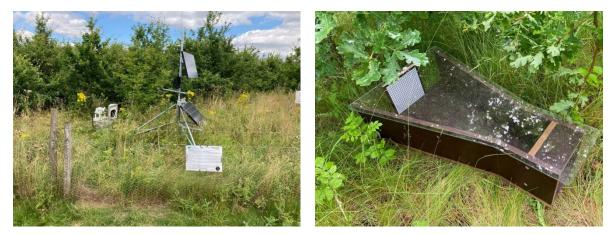
Figure 16: Autonomous biodiversity monitoring station on the lineside (left), Small mammal camera trap (right), © Network Rail
