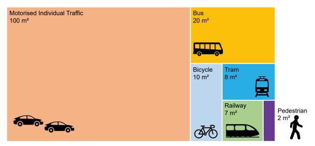
Figure 1: Land consumption by mode of transport in square metres per person transported in urban transport (Ref e: Allianz pro Schiene, 2020)
