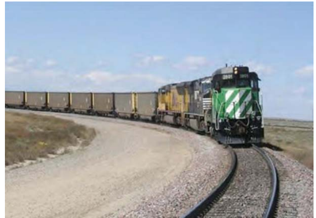
Figure 3. Photograph of the Heavy Axle Load Train at the Facility for Accelerated Service Testing at TTC.
