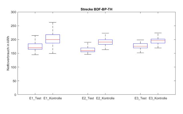
The energy consumption in suburban railway operation can be reduced by up to 10-15% if,
