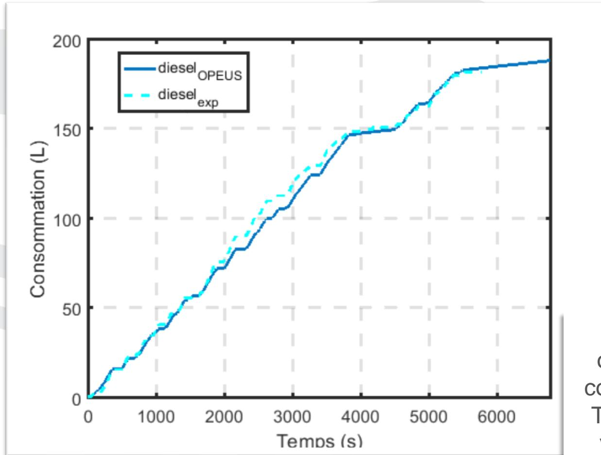
The simulation overestimates the consumption by 1%. The OPEUS tool is validated from an energy point of view.
