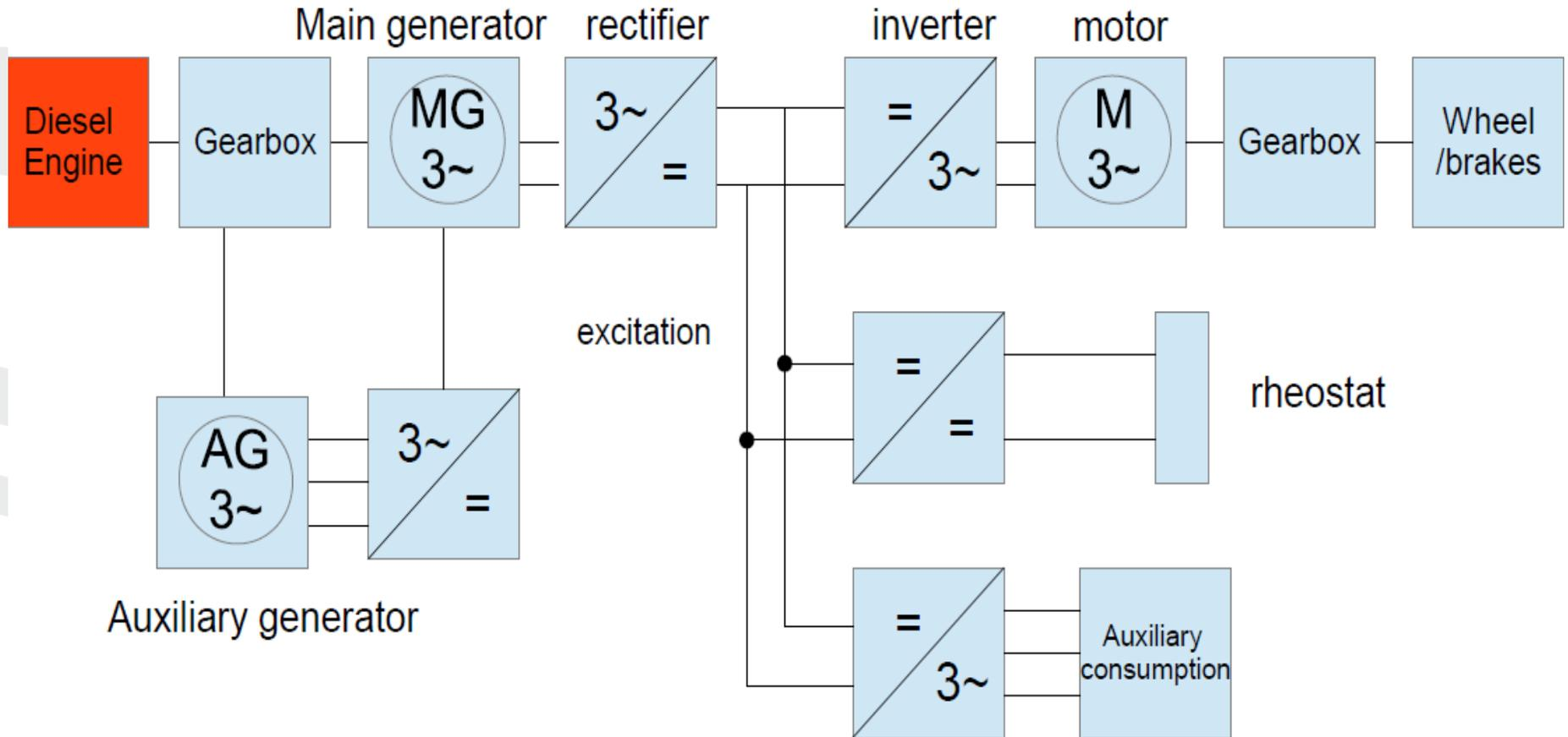
Diesel electric traction
