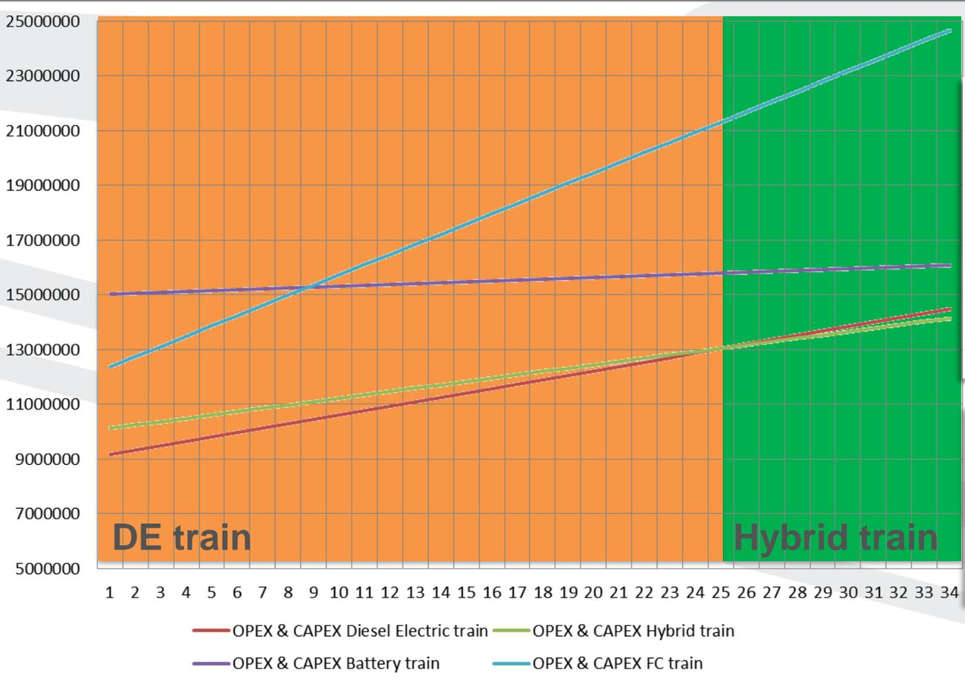
The diesel electric train seems to be the most relevant one during the first years.
