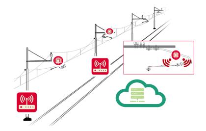
Use of low-cost transducers that can be integrated into the material (<u>Smart Material</u>) and sensor nodes with Computational Capacity for Structural Monitoring tasks with selffeeding systems (<u>Harvesting</u>)
