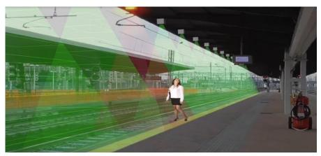
With the innovative intrinsically safe radar technology, a system is set up **to monitor passenger behavior** while waiting for the train, in order to prevent actions such as crossing the track. Power Supply
