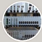
ON BOARD ATP ATO SYSTEM
