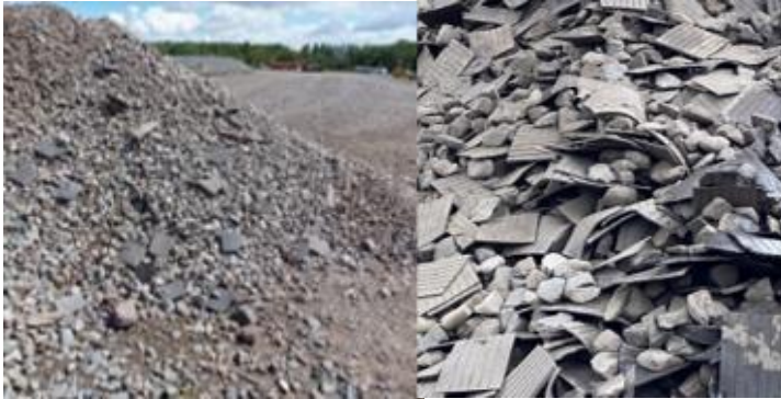
Figure 16 : used pads mix with ballast
