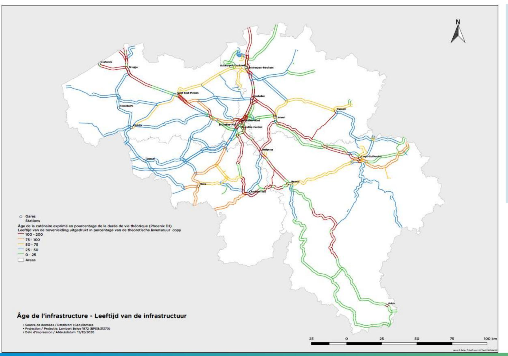
**Renewal Strategy OCL & substations** After 20 years  $\rightarrow$ mid-life upgrade substation After 40 years  $\rightarrow$ renewal substation →mid-life upgrade OCL After 60 years  $\rightarrow$  mid-life upgrade substation After 80 years  $\rightarrow$ renewal substation  $\rightarrow$ re-electrification with OCL ? Partly ??
