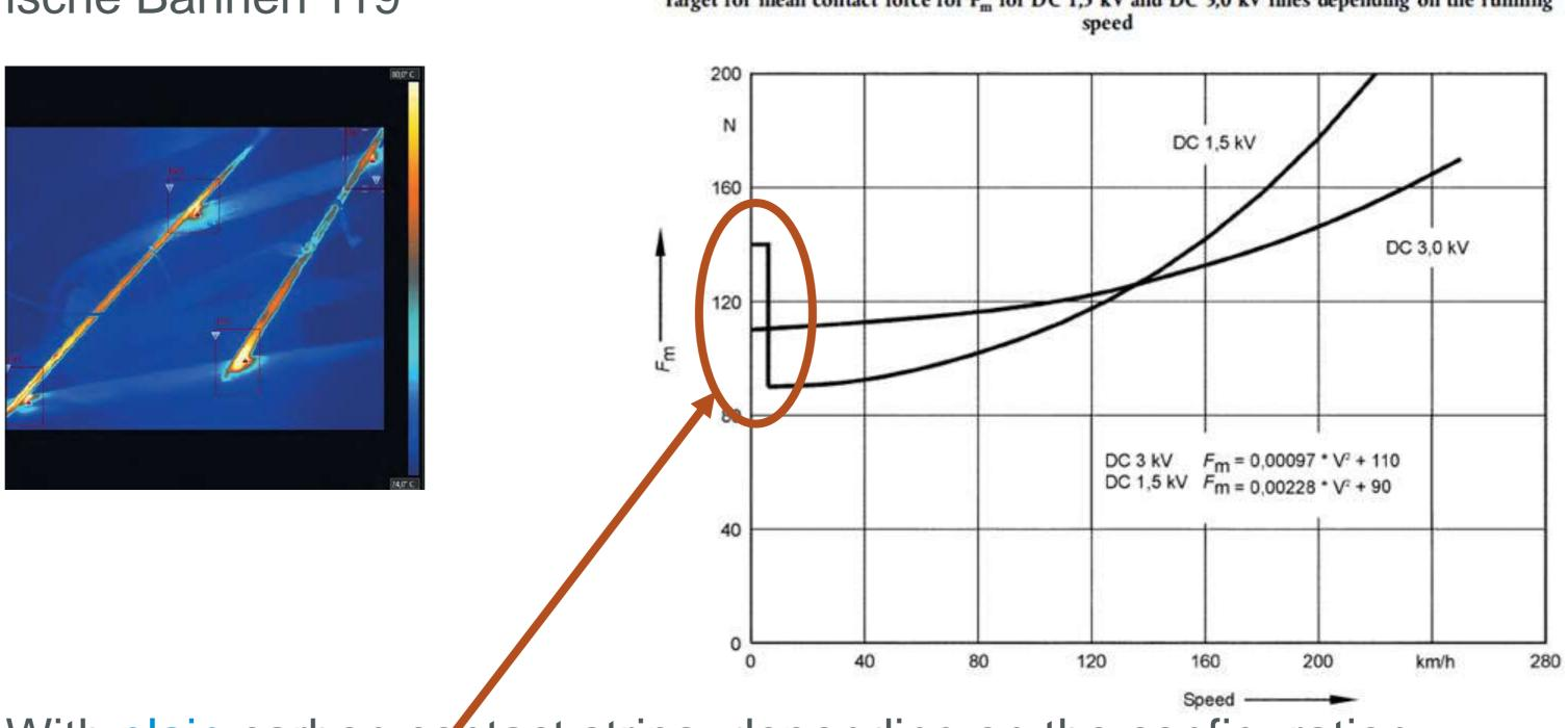
With <u>plain</u> carbon contact strips, depending on the configuration: - 140N static contact force instead of 70N as usual in AC systems - 2 rigid OCLs with a CuAg 120mm<sup>2</sup> wire, spaced 40 cm apart it is possible to go from the actual legal 80A to 220A !  $\rightarrow$  3,3 MW under 15kV AC → 5,5 MW under 25kV AC !
