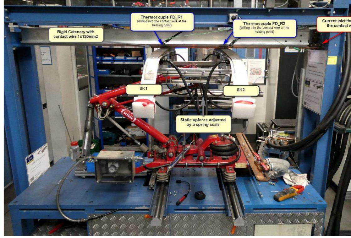
Test bench Schunk (SK2488-a), with a short rigid catenary & 1x120mm<sup>2</sup> contact wire
