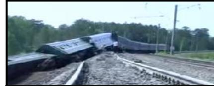
Derailed on the Shimanovskaya – Seletkan line caused by cryogenic processes
