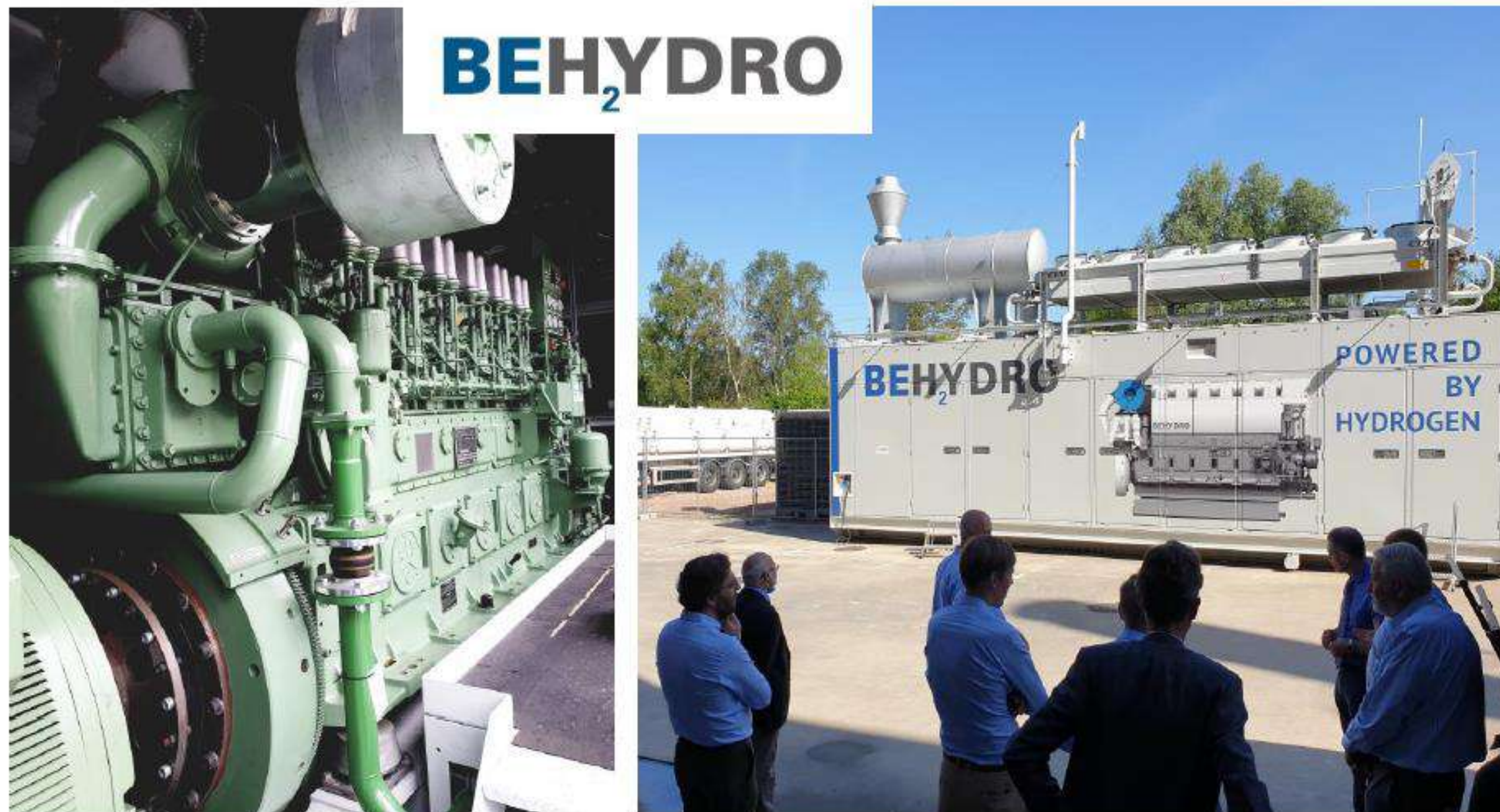
Medium speed hydrogen engines are based on the proven DZ series from ABC engines
