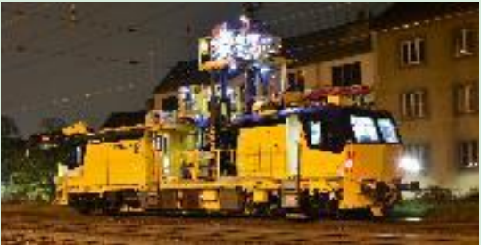
MTW 100 Catenary inspection
