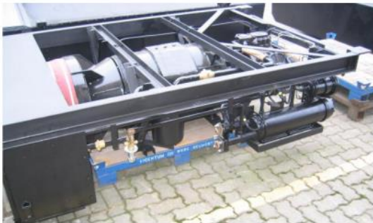
HVAC saloon installed on the underframe
