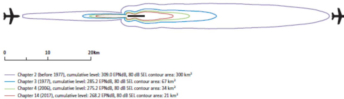
Figure 2.2 80 dB Sound Exposure Level (SEL) contours for different aircraft that just meet the various ICAO Chapter limits
