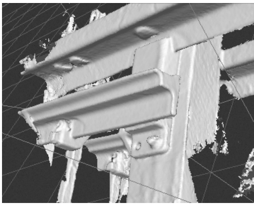
Fig. 2. Undamaged UIC60 switch blade in 300 radius 3Dmodel scanning by Kinect device
