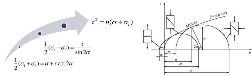
(1) the gradient of curve decreases with the increase of stress, and (2) the friction angle becomes smaller as it is concerned with the nature of undisturbed loess itself.
