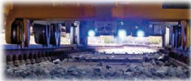
Optical measurement of track geometry
