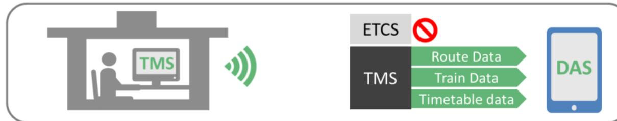
For C-DAS, IM should deliver extra train, infra, timing and communication data
