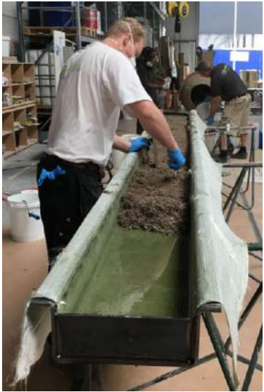
Production of deck profiles with re-used EoL composite
