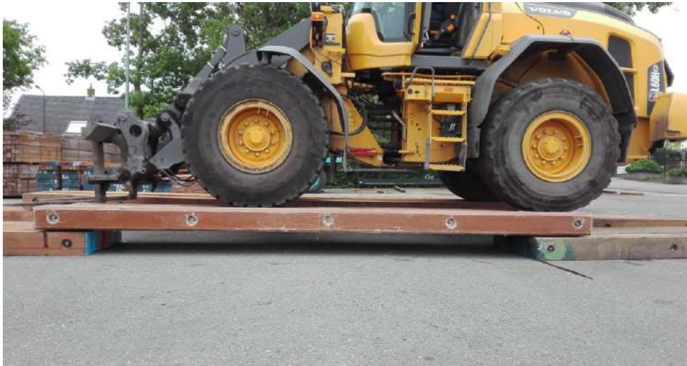
Crane mat test with heavy vehicle
