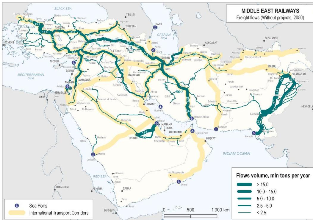
**Figure 46. Modelled rail flows in the Middle East region by 2050 under baseline scenario with ADDITIONAL LINKS (suggested projects)**
